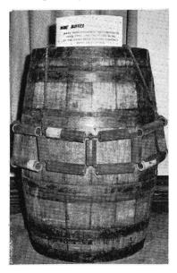
Wine cask with buffers. Made from discarded Westinghouse hose pipes, they protect the casks from damaging contact with each other.
