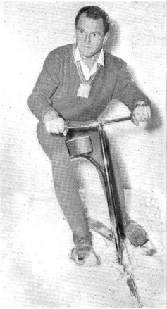
The latest: Mr. Ollie Polasek shows how the bicycle is used. Europe's latest snow sport craze, the has a fixed ski at the rear and a moveable skiby handle-bars—at the front. The rider uses skis to assist control as the bicycle speeds down slopes. It makes its first public appearance at The Mt. Buffalo, this season, where Mr. Polasek is an in
