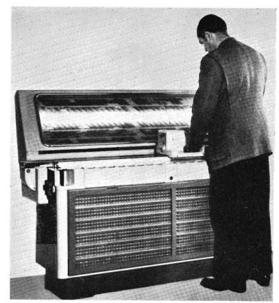
Operator moves the carriage to select a printing plate. At the present time, no machines of this type are operated in Australia, but they are extensively used in Great Britian and on the Continent.
